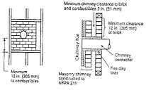
Minimum chimney clearance from masonry to sheet steet supports and combustibles 2 in, (51 mm)
